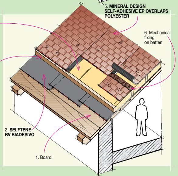
wooden boarding etc., the surface to be covered should be prepared with a coat of 250 or 500 g/m<sup>2</sup> INDEVER PRIMER E primer, which is also recommended on metal surfaces.
